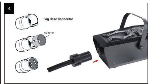
Attach the other end of the (E) Fog Hose to the fog machine as shown in Figure 4.
